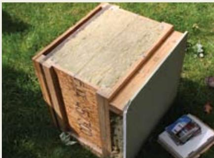
**page 3** Sample of the super insulated wall construction
