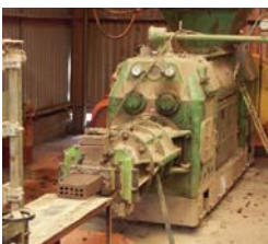
Top: making the unfired bricks. Bottom: building with unfired bricks All images ©Arc
